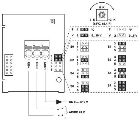
The adjustment of the measuring ranges is made by changing the bonding jumpers. The output value in the new measuring range is available after 2 seconds.
