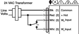
Floating Point - Triac Source 24 VAC Transformer Blk (1) Common Red (2) + Hot Wht (3) W<sub>3</sub> Input Wht (5) W₄ Input
