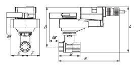
Weight [kg] Type DN [kg] B280 80 4.1 C D H1 В Ε F H2 11.0" [280] 8.5" [217] 2.8" [71] 5.8" [148] 6.0" [152] 2.8" [71] 2.1" [53] 0.8" [20]
