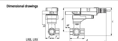
Type DN Weight [kg] [kg] B318B 20 0.40 Ε В C D F H1 H2 8.5" [216] 2.7" [69] 5.8" [147] 5.1" [129] 1.3" [33] 1.5" [39] 1.2" [30] 1" [25]
