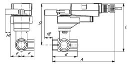
Type DN Weight [kg] [kg] B320B 20 0.50 C Ε В D F H1 H2 8.5" [216] 2.7" [69] 5.8" [147] 5.1" [129] 1.3" [33] 1.5" [39] 1.2" [30] 1" [25]
