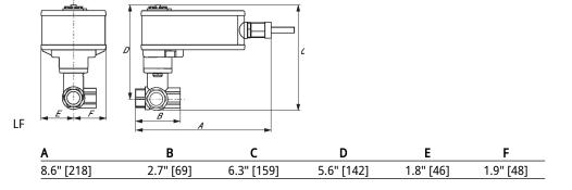
Modulating, Non-Spring Return, 24 V, for DC 2...10 V or 4...20 mA
