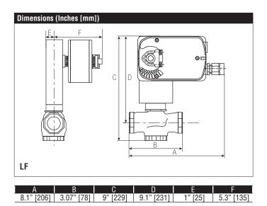
LF24-MFT US, Valve Actuator Modulating, Spring Return, Multi-Function Technology®
