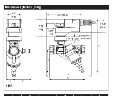
LF24-MFT US, Valve Actuator Modulating, Spring Return, Multi-Function Technology®
