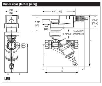
LF24-MFT-S US, Valve Actuator Modulating, Spring Return, 24 V, Multi-Function Technology®
