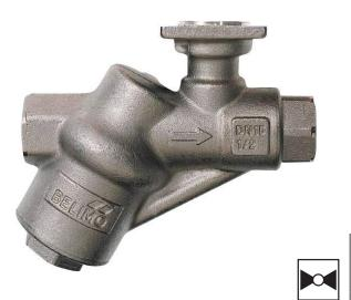
Application The Pressure Independent Characterized Control Valve is typically used in air handling units on heating and cooling coils, and fan coil unit heating or cooling coils. Some other common applications include unit ventilators and VAV reheat coils. This valve is suitable for use in a hydronic system with constant or variable flow. This valve is designed with MFT functionality which facilitates the use of various control input.
