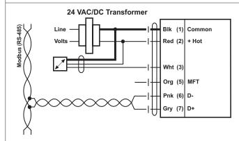
Modbus control with active sensor for Non-Spring Return
