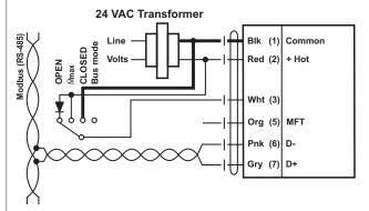
Modbus control with local override (AC only, analogue override) for Non-Spring Return
