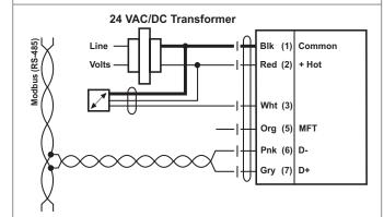
Modbus control with active sensor for Non-Spring Return
