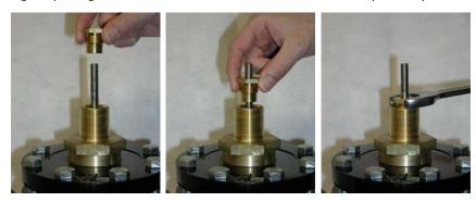
Step by step procedure for removal of existing v-ring or lip packing & installation of lip packing repack kit.
