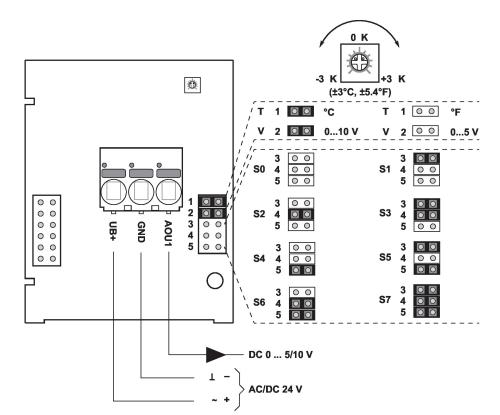
The adjustment of the measuring ranges is made by changing the bonding jumpers. The output value in the new measuring range is available after 2 seconds.
