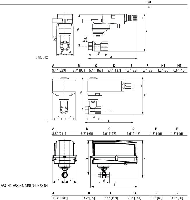
NEMA 4X, Modulating Control, Non-Spring Return, 24 V, for DC 2...10 V or 4...20 mA
