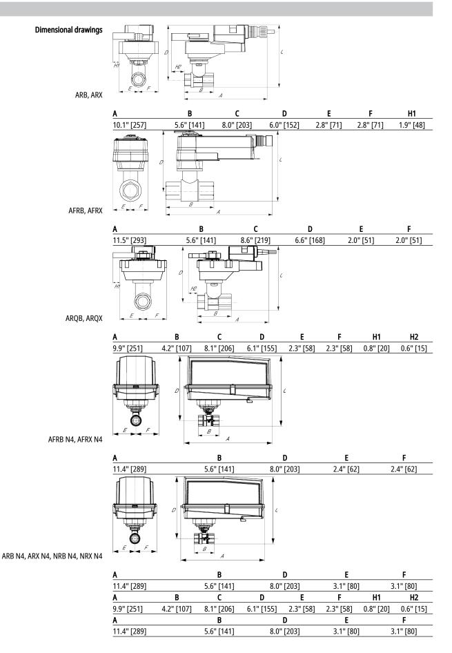
On/Off, Floating Point, Non-Spring Return, AC 100...240 V
