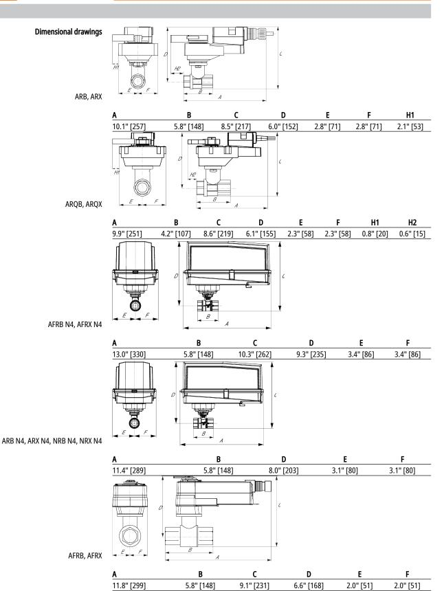
On/Off, Floating Point, Non-Spring Return, AC 100...240 V
