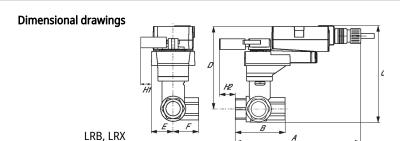
Type DN Weight [kg] [kg] B309B 15 0.30 Ε В C D H1 H2 1.1" [28] 8.5" [216] 2.4" [60] 5.2" [132] 4.6" [117] 1.3" [33] 1.3" [33] 1.2" [30]
