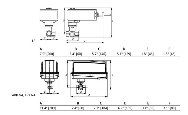
Modulating, Non-Spring Return, 24 V, 0 to 135  $\Omega$  Input
