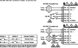
Multiple Actuators with Minimum Position Potentiometer
