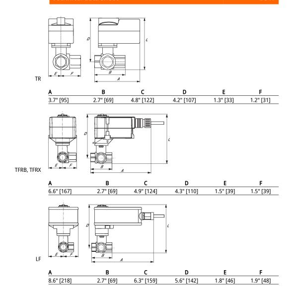
Modulating, Non-Spring Return, 24 V, for DC 2...10 V or 4...20 mA
