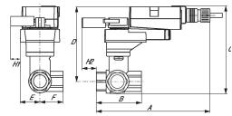
Type DN Weight [kg] [kg] B321B 20 0.50 C Ε В D F H1 H2 8.5" [216] 2.7" [69] 5.8" [147] 5.1" [129] 1.3" [33] 1.5" [39] 1.2" [30] 1" [25]
