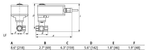
On/Off, Spring Return Fail-Safe, AC 120 V
