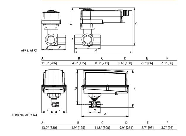
NEMA 4, Modulating Control, Non-Spring Return, Direct Coupled, 24 V, Multi-Function Technology®
