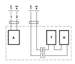
A = Actuator T [°C] = Thermostat H = Heating
