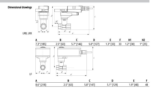
On/Off, Spring Return Fail-Safe, AC 120 V
