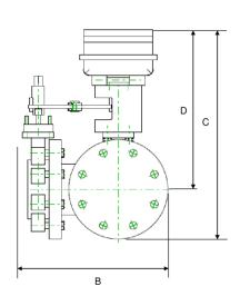
Modulating, Non-Spring Return, 24 V, for DC 2...10 V or 4...20 mA
