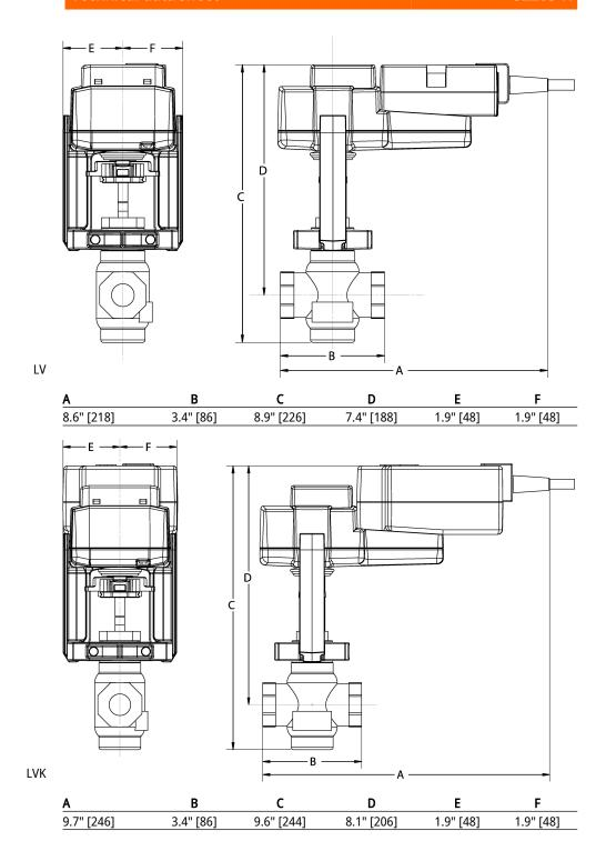
On/Off, Spring Return Fail-Safe, AC 120 V
