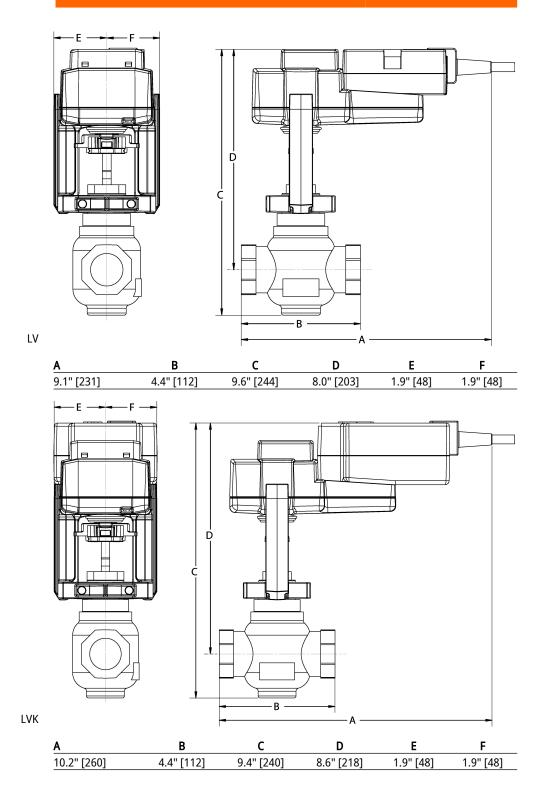
On/Off, Spring Return Fail-Safe, AC 120 V
