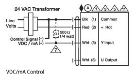
24 VAC Transformer (AC Only) Blk (1) Common Red (2)+ Hot Wht (3) Y Input Position (-) Feedback VDC (+) **U** Output
