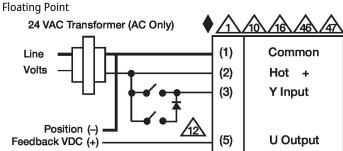
VDC/mA Control **1**√3√5√16√46 24 VAC Transformer (1) Common Line Volts (2) Hot + 500 Ω 1/4 watt Control Signal (-) VDC/mA (+) (3) Y Input Position (5) **U** Output Feedback VDC
