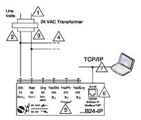
Initial ethernet connection and set-up
