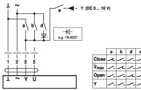
Override control and limiting with DC 24 V with relay contacts
