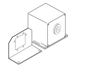
4 Match the hole pattern of the shaft face to the existing linkage and utilize the #6-32 screws and nuts with the ECON-ZIP-ACT to secure into place. **Note: At least 2 screws and nuts should be used**.
