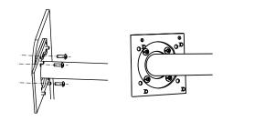
5 Slide the actuator onto the shaft, Secure the actuator to the mounting plate with the two 1/4-28 screws and nuts provided.
