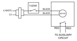
Built-in Auxiliary Switch (optional) (only on -S models)
