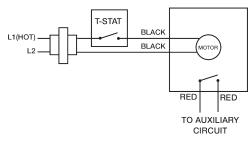
Built-in Auxiliary Switch (optional) (only on -S models)
