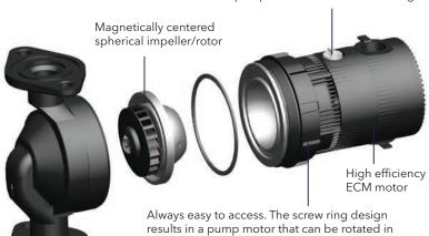
results in a pump motor that can be rotated in any position around the 360° circle. Therefore the electrical connection as well as the control dial is easy to access.
