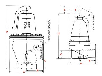
MODELS 3301 AND 4100 Iron body relief valves are not recommended for use on domestic water service.
