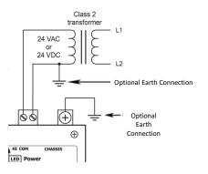
**WARNING:** Internally, this device utilizes a half-wave rectifier and therefore can only share the same AC power source with other half-wave rectified devices. Sharing a common DC power source is also possible. Sharing AC power with full-wave rectified devices is NOT recommended. Devices powered from a common AC source could be damaged if a mix of half-wave and full-wave rectified devices exists.
