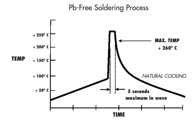
The above flow-wave soldering profile applies to all CR8300 and Custom CR8400 PCB Mount Current transformers.
