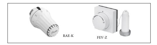
The RAE-K and FEV-Z styles of thermostatic operators provide an effective use of pressure independent flow control with a non-electric control valve. By using the ABQM pressure independent control valve (PICV) proper flow is maintained to the emitter. With the thermostatic operator mounted to the valve, a cost effective method of control is used to maintain the room temperature.
