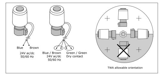
When 24 volts is applied to the actuator, the internal wax element heats up allowing the valve to actuate. Unlike valves that open and close quickly, the actuation of the TWA is slow, reducing water hammer and as a result performs similar to a modulating valve in certain situations.
