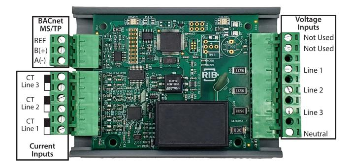
**CONNECTING MULTIPLE LOADS:** The RIBPM413-BC allows for multiple loads to be metered at once, by
