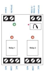
\*Must clip resistor in white box for 0-5Vdc.
