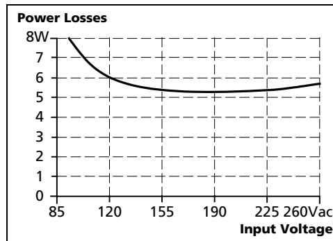
Fig. 8-4 Losses vs. input voltage at 24V, 2.5A, typ.
