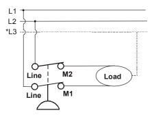
Line to M1, and Line to M2 open on pressure rise.
