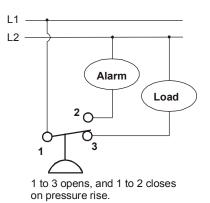
Figure 6: Typical Wiring for SPDT Switch (P70E, F Models)
