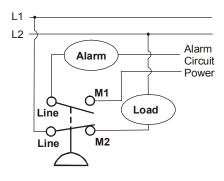
Main circuit (Line to M2) opens and auxiliary circuit (Line to M1) closes on pressure rise.
