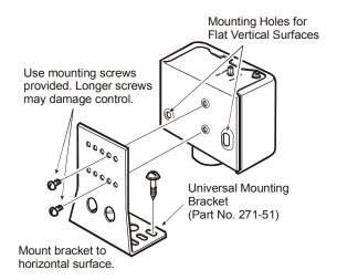
Figure 4: Mounting the P70, P72, and P170 High Pressure Control with NEMA 1 Enclosure
