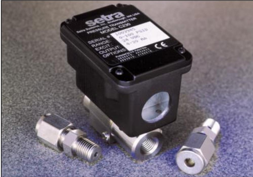
Setra Systems Model 230 is a high output, low differential pressure transducer designed for wet to wet differential pressure measurements of liquids or gases. A fast-response capacitance sensor and signal conditioned electronic circuitry provide a highly accurate, linear analog output proportional to pressure. Both unidirectional and bidirectional pressure ranges are available for applications with line pressure up to 250 psig.
