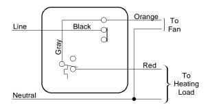
Figure 6: T46ADH Off-Auto Selector Switch with Continuous Fan (Heating Only)
