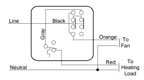
Figure 7: T46ABH Auto-Off-Fan Selector Switch with Continuous Fan (Heating Only)
