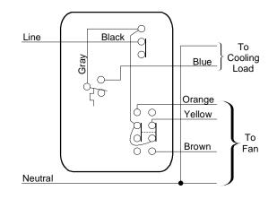
Figure 10: T46JEA On-Off Selector Switch with Fan Speed Control (Cooling Only)
