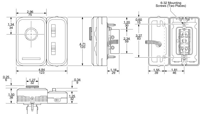
Figure 4: T46 Dimensions (in./mm)
