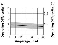
Figure 2: Operating Differentials for T46A and Heating Side of T46S
