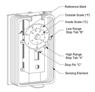
Figure 16: T46 Thermostat Range Tabs and Stop Pin
