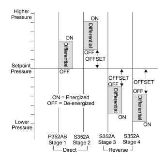
Figure 8: Example of a Reverse Acting/Direct
