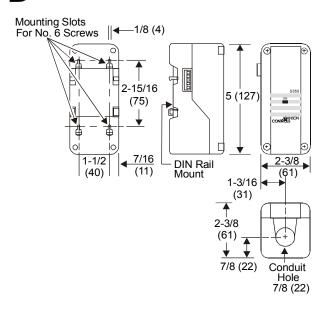
Figure 2: System 350 Stage Module Dimensions, in. (mm)
