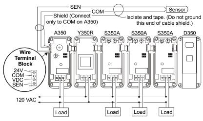
Figure 9: Typical Multistage Temperature Control System Using 120 VAC Power Supply
