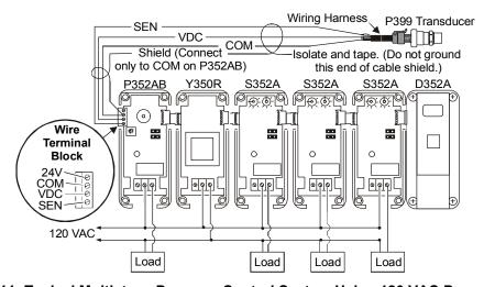
Figure 11: Typical Multistage Pressure Control System Using 120 VAC Power Supply
